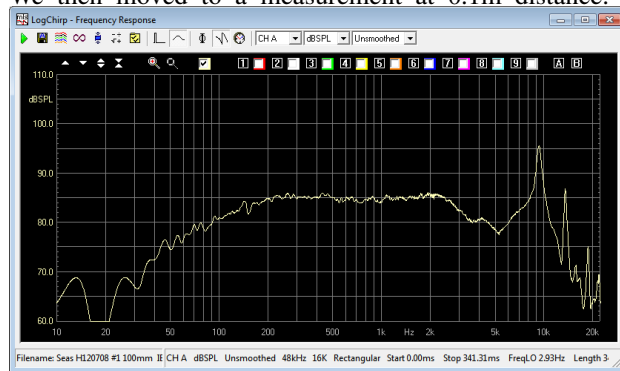
Figure 10. H1207 on Large IEC Baffle measured at 100mm.
