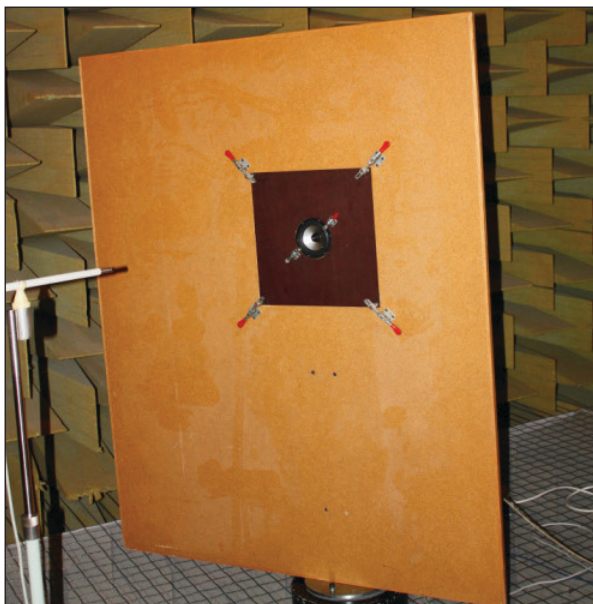
Photo 3: A SEAS anechoic chamber is used to take a comparative International Electrotechnical Commission (IEC) baffle measurement.
