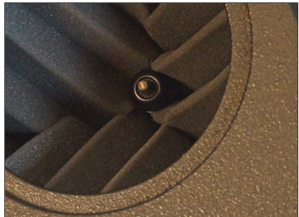
Photo 5: This is a close up view of the microphone mounting location in the Hill Acoustics TTC 350.
