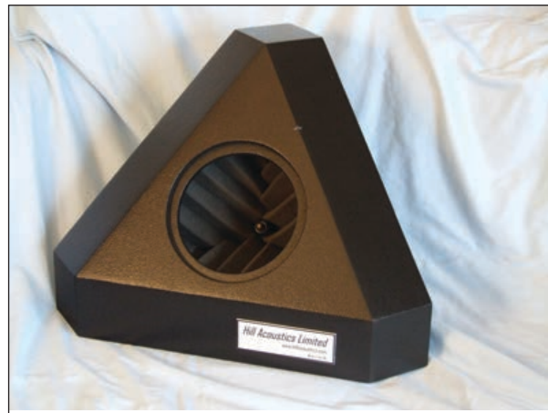
Photo 4: The Hill Acoustics Tetrahedral Test Chamber (TTC) 350 is a mini anechoic chamber that is said to produce consistently accurate results.
